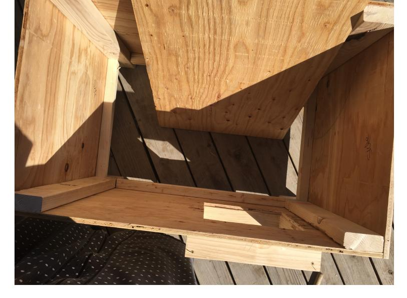
Screw the 38.5" and 23.5" 2x2's around the edge of the roof board to make a rim.
